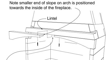
Mortar arches in place and drill Ø1/8" pilot holes into lintel. Secure arches with 1/4" Tapcon screws.
