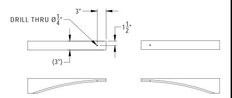
Arch is made for 49" unit. If used in smaller models, cut down to size needed.
