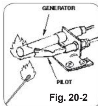
**Note:** Pilot flame should encircle tips of the electrodes.
