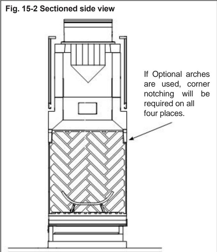
firebrick or the firebrick mortar performs. It is not unusual in the course of the life of the firebrick, or the firebrick mortar, for heat stress cracks to appear. Burntech® cannot be responsible for this and other wear and tear to the firebrick and mortar.
