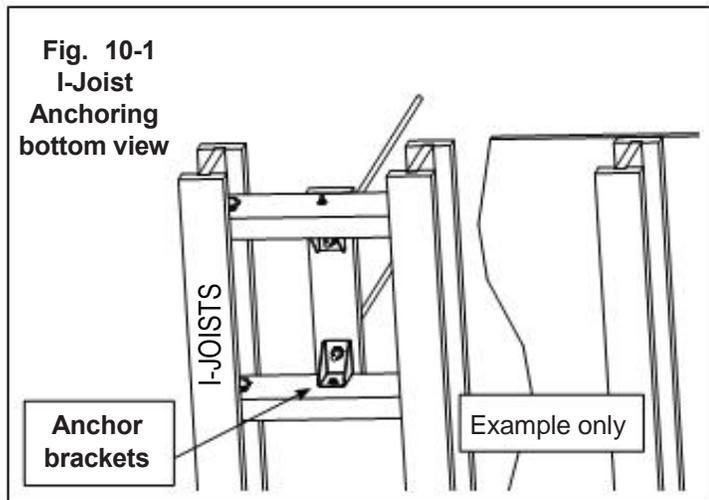
For installation of firebox over combustible crawl spaces or upper floors, anchorage of the firebox is required. Illustrations of examples of possible anchorage methods are shown in Fig. 9-2 thru 10-2 depending upon the type of floor framing. Final method of anchorage to be determined by licensed design professional.
