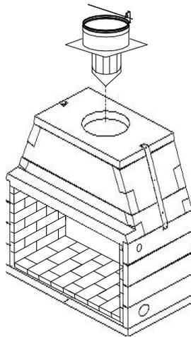
**Attention:** Clearance to combustible construction can not be reduced during course of construction. For safe operation of the finished fireplace, these clearances must be followed when building the framework to house the chimney system.
