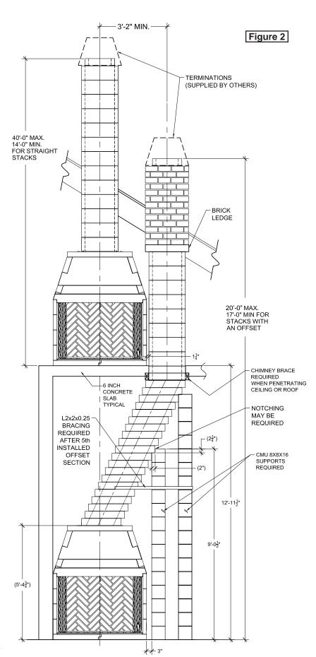
The Burntech Masonry Chimney System consists of the
