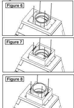
5. If an offset is required after a short run of straight fl ue, start with a standard 8" high inner flue (MCH-814). The offset will require that the inner and outer flue is flush at the beginning of the offset sections. After the offset is complete, resume the straight stack with a short 4" high inner fl ue (MCH-414) and continue with 8" high inner and outer sections (MC H-814, MCH -814). At the point
