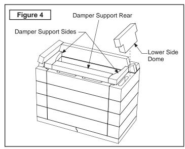
Install Damper System per its' manufacturer's instructions. Some systems come with pre-drilled holes for securing with Tapcon® screws.
